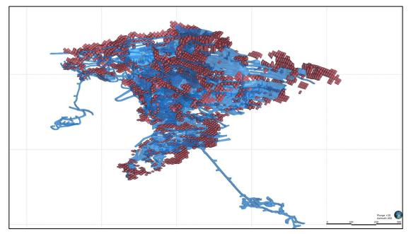
Figure 1-1: North east view of the MSO shapes (red) in relation to the depletion survey (blue). The MSO shapes are used to constrain the reporting of the Mineral Resources.
