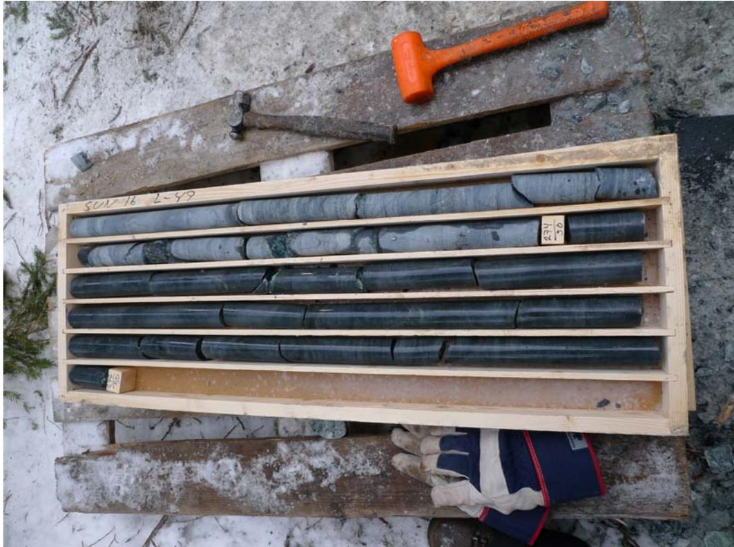
**Figure 11-1: Typical example of drill core quality in Serpentine from the Project area. (Photo represents core from hole 16 at a depth of 275m, Sundsberget.)**
