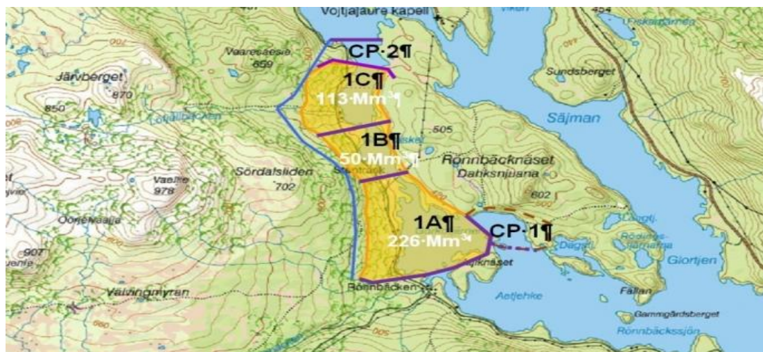
Figure 18-2: Proposed design layout of the Rönnbäcken TMF
