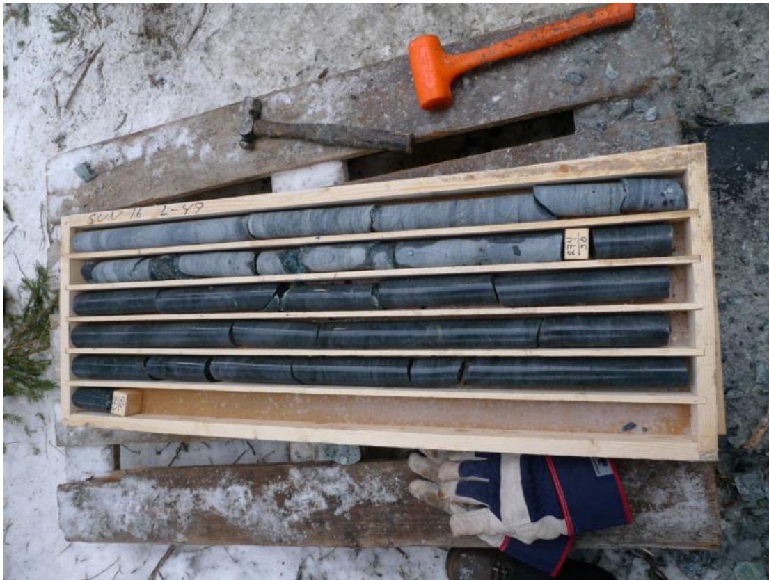
Figure 11-1: Typical example of drill core quality in Serpentinite from the Project area (Photo represents core from hole 16 at a depth of 275 m, Sundsberget)
